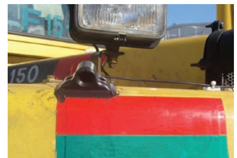
Cameras installed on forklifts
